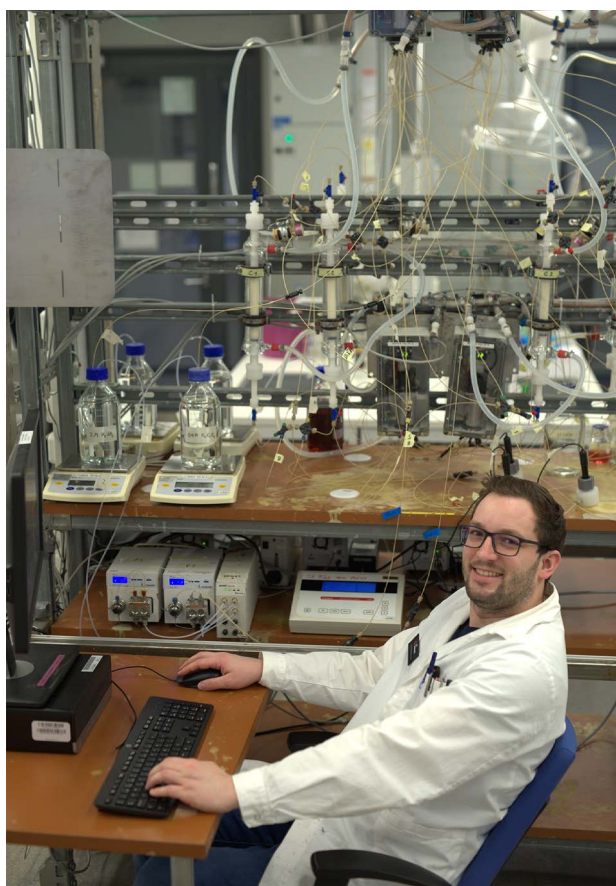
Fig 1. Tobias Wesselborg in running simulated moving bed experiment for his PhD work with LUT's self-designed and -built (under Prof. Tuomo Sainio) continuous ion exchange workstation.
