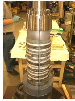
Magnets Epoxy Bonded to Shaft @ AT Lab
