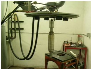
Precision Balanced and Spun Tested to 33,000 rpm, 150 C @ The Balancing Company, OH
