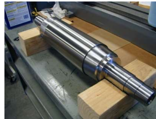
Final OD Grinding @ UniGear, Canada
