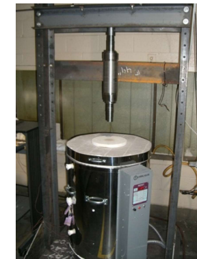
IN718 Sleeve Shrunk Fit onto Rotor (1200 F, .025in Interference), Special Press and Furnace built @ RGG, GA
