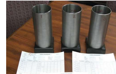
IN718 Sleeves Formed, Machined, Heat Treated and Final Grind @ FlowTurn, OH
