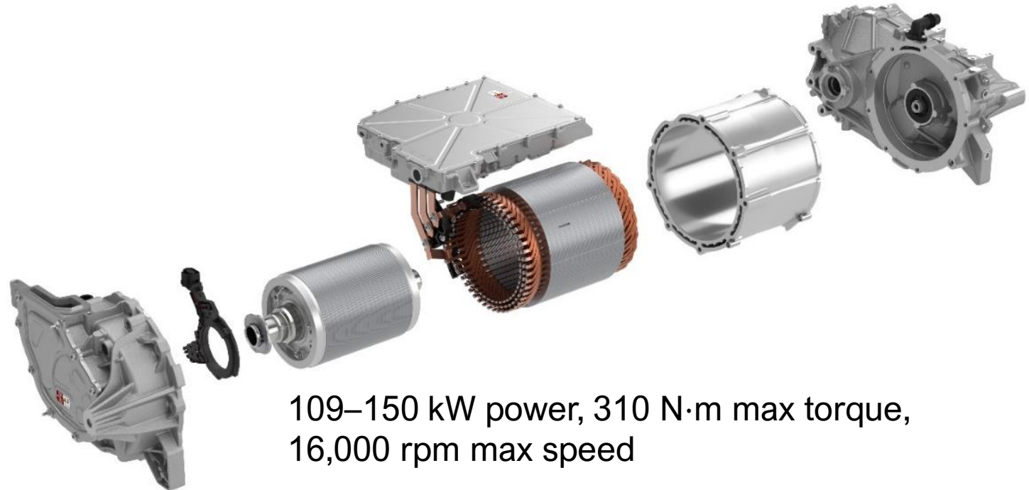
Rear-axle 8-pole PMSM
