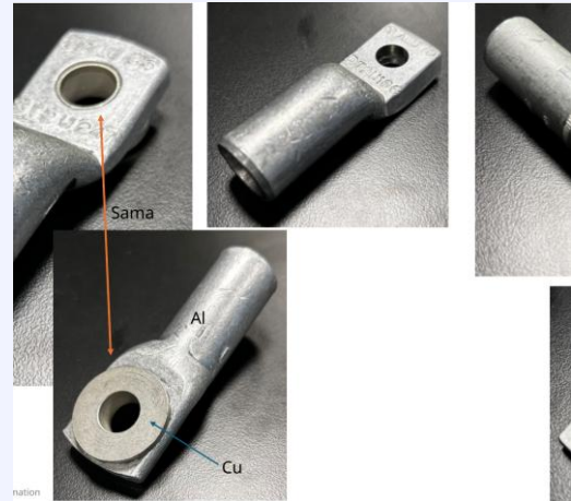
Example connector candidates and bi-metallic interfaces reviewed for aluminum cables and busbar connections.
