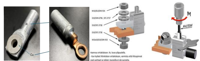
Preliminary Results: Connector designed for aluminum cables and copper connections, great economic importance
